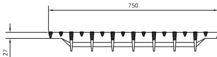
Made of ductile iron. Fulfils the requirements of European standards EN-124.
