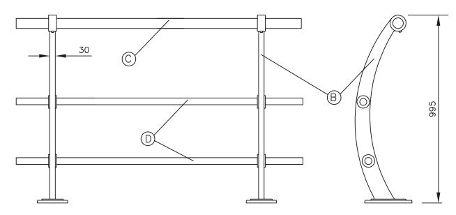
MATERIAL: B.— 1000mm. iron post. C.— Ø51mm stainless steel tube.
